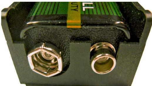
**Insert the battery – Be careful to make sure its in the correct way !
