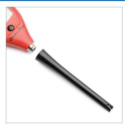
The HI1271 pH electrode can be easily replaced. Just unscrew the electrode from the meter body and screw on a new one.
