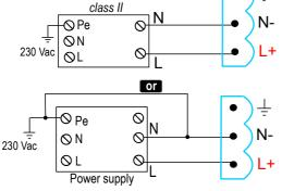
For transmitters with 115 or 230 Vac power supply:
