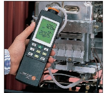
Checks gas flow pressure
