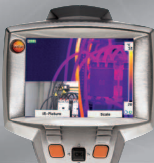
Image-in-image function for easier orientation and simple documentation
