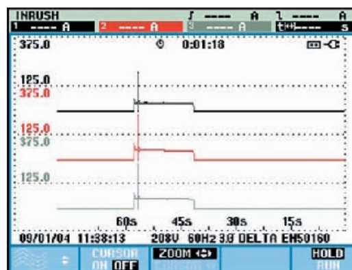
Inrush function automatically triggers off of current, and captures start up measurements on motors and other devices to help determine trip levels.
